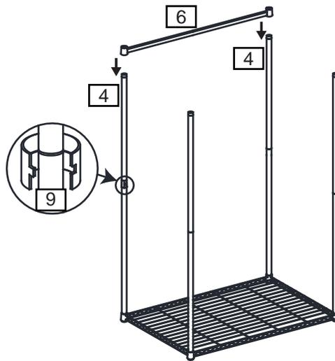
b: Attach shelf [3] and the plastic holder [9] to thin rods [5] as shown
