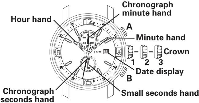
A chronograph combines two time-keeping functions: In addition to indicating the time on its dial, a chronograph can also be operated like a stopwatch to measure intervals of time.
