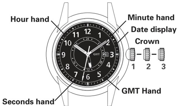
NOTES: Setting the Hour hand on the exact hour provides the most accurate time setting. If the Hour hand is set between hours, it may prevent the time from being accurately displayed and read.
