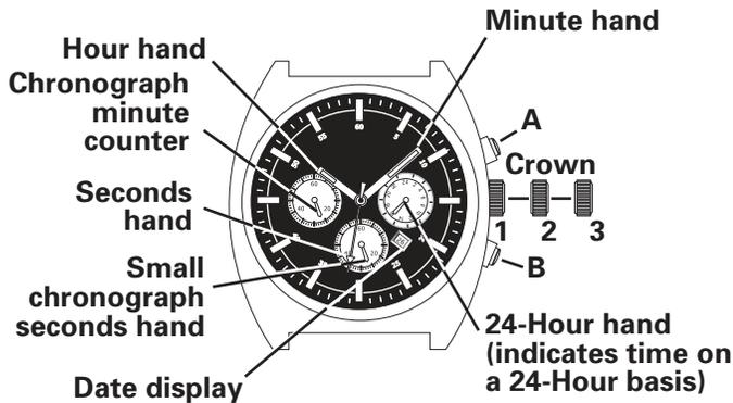
This chronograph can be used to time events up to 59 minutes/59 seconds in duration, in whole second increments.
