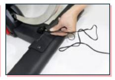
Plug power adapter into port located on the rear foot bracket, then plug into wall outlet.
