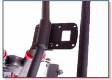
Ensure wires are still pulled out and insert post into the frame while pulling out handlebar adjustment lever.
