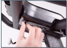
Attach back of console to handlebars by inserting screws and finger tightening.
