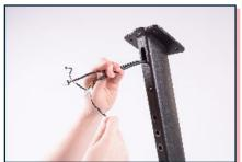
Make sure to pull out enough length Unwrap the twist tie and separate the wires.
