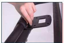
While holding handlebars in place, insert bolts and finger tighten.
