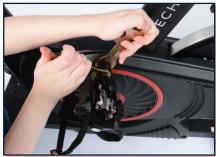
Hold pedal with double sided wrench and use single sided wrench to tighten nut counterclockwise.
