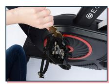
Screw left pedal onto crank arm counterclockwise. Use double sided wrench to ensure pedal is firmly seated against crank arm.
