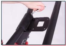
Use included hex key to tighten and secure handlebars in place.
