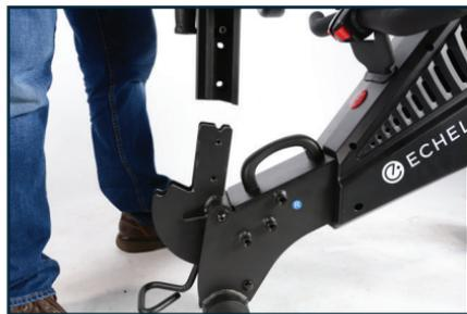
7. Place the rail onto rail bracket.
