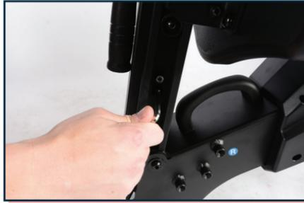
9. Tighten screws with hex key.
