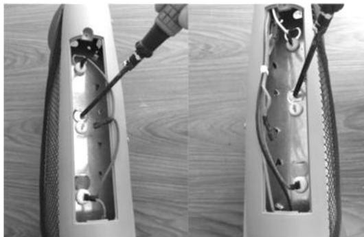
1. Reconnect the wires to the tube terminals on both sides.
