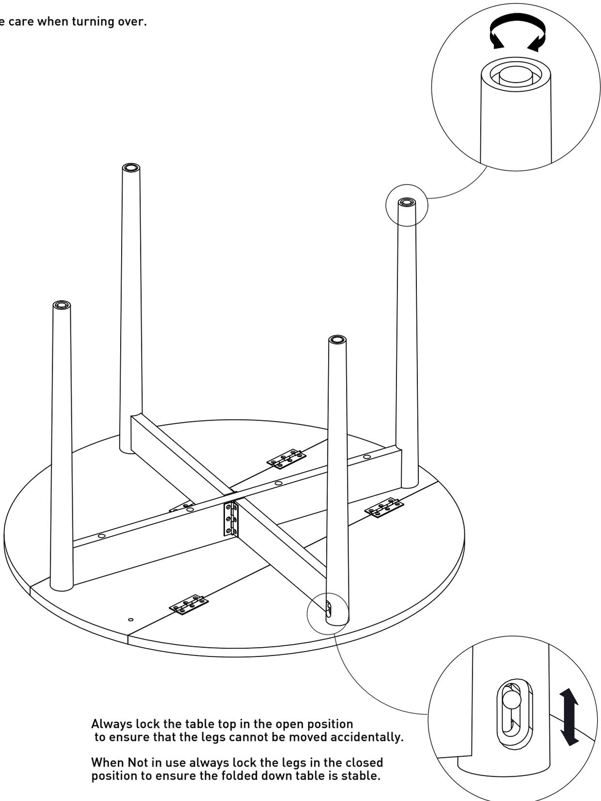
Always lock the table top in the open position to ensure that the legs cannot be moved accidentally.
