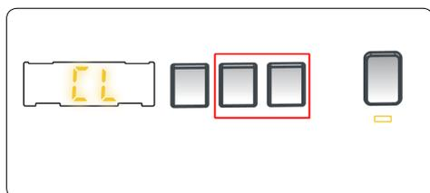
If any button is pressed or the selected programme is changed by the programme dial while the child lock is active, the "CL" symbol will flash on the electronic display for 2 seconds.
