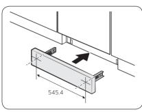
2. Insert the pre-cut skirting board into the brackets first, and then tighten the screws to fix the board. See the figure on the left and make sure the brackets are positioned in the correct place.
