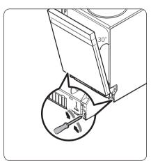
**14.** Adjust the spring level while the door is approximately opened at 30 degrees. The door should hold its position, and should not fall open.
