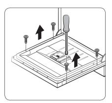
9. Open the dishwasher door and remove the 4 screws.
