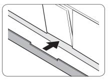
4. Attach the cut skirting board to the bottom of the dishwasher. Make sure the board does not interfere with the door of the dishwasher.
