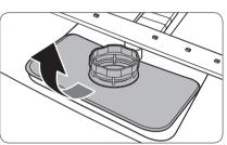
**3.** Remove the Coarse filter, and then the cylindrical micro filter underneath.
