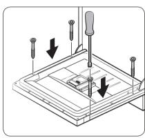
**10.** Secure the custom panel to the door by fastening the 4 screws (Ø3.5 X 45).
