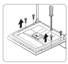
12. Open the dishwasher door and remove the 4 screws.
