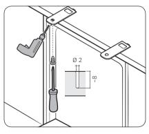
3. Tighten the 2 screws (Ø4 X 14) to fix the brackets.
