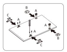
3. Remove the installation template, and then tighten the Custom panel fixers (B), (C) with 12 screws (A) as shown in the figure.
