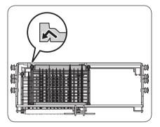
**2.** Gently lift the left shaft of the tray and move up to the opening hole of the chassis.
