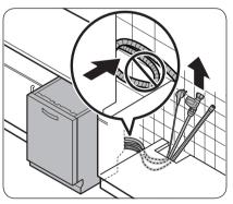
**3.** Pull the power plug, the water hose, and the drain hose through the sink hole.
