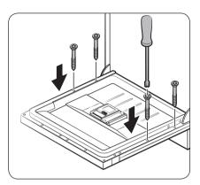
**13.** Secure the custom panel to the door by fastening the 4 screws (Ø4 X 43).
