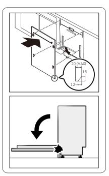
**4.** While holding the custom panel, attach it to the door and insert the Custom panel fixers into the corresponding holes at the door.
