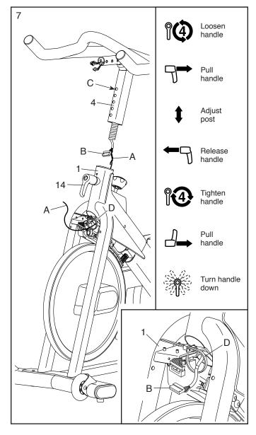
8. **See the inset drawing.** Connect the connector on the Upper Wire (B) to the connector on the Lower Wire (82).
