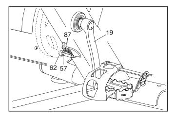
Next, turn the Left Crank Arm (19) until a Magnet (62) is aligned with the Reed Switch (57). Slide the Reed Switch slightly toward or away from the Magnet. Then, retighten the M4 x 20mm Screws (87).
