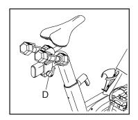
Note: The carriage handle (D) functions like a ratchet. Turn the carriage handle in the desired direction, pull it outward, turn it in the opposite direction, push it inward, and then turn it in the desired direction again. Repeat this process as many times as necessary.
