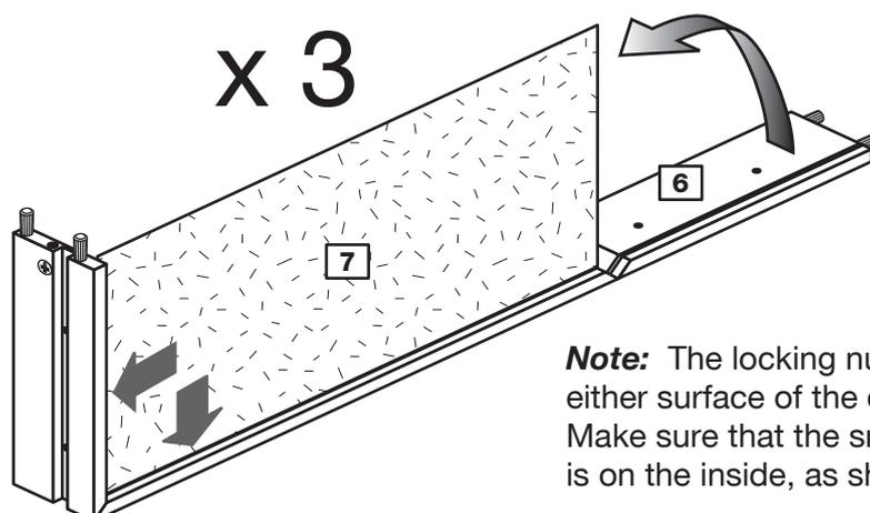
**Note:** The locking nuts can be on either surface of the drawer sides. Make sure that the small groove is on the inside, as shown.
