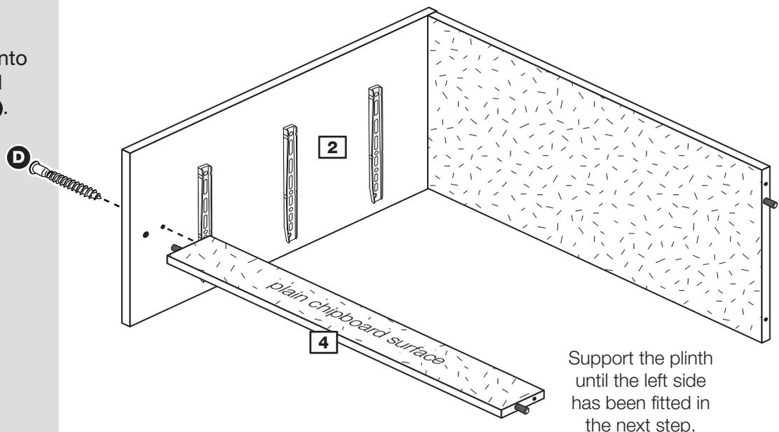
Support the plinth until the left side has been fitted in the next step.
