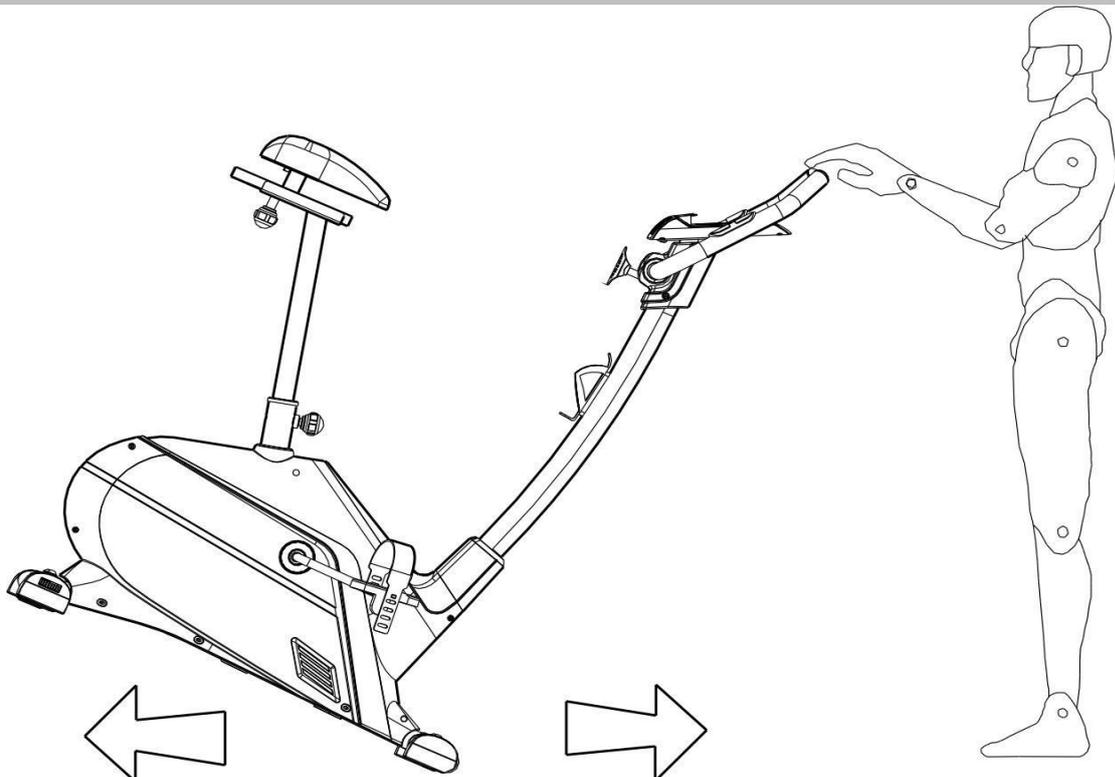
Hold the handle to move the bike as shown in the diagram.
