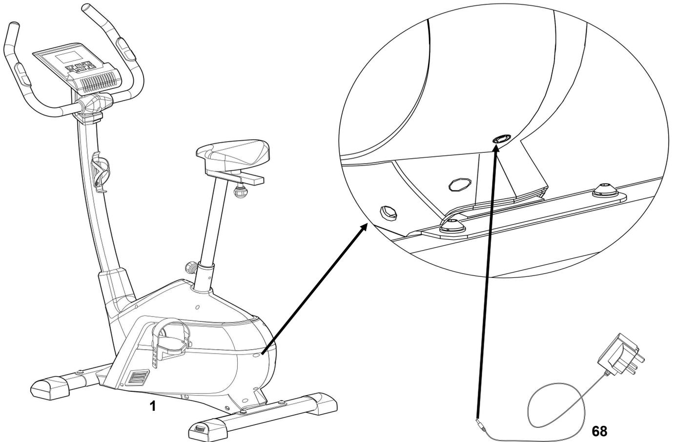
Insert the power Charger (68) into the hole on the Main Frame (1) as shown in the diagram.
