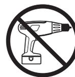
• We do not recommend the use of power drill/drivers for inserting screws, as this could damage the unit. Only use hand screwdrivers.
