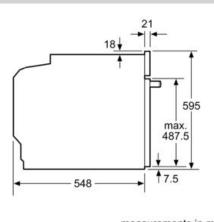
measurements in mm
