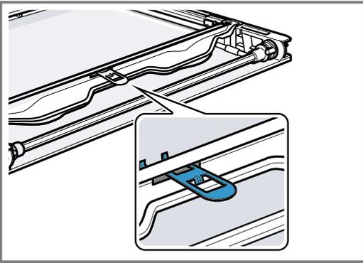
✓ The retainer has been inserted.
