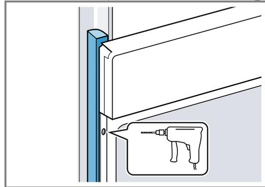
3. Secure the appliance using a suitable screw.
