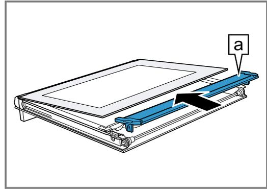
8. Insert the inner pane with the holder **a** into the opening.
