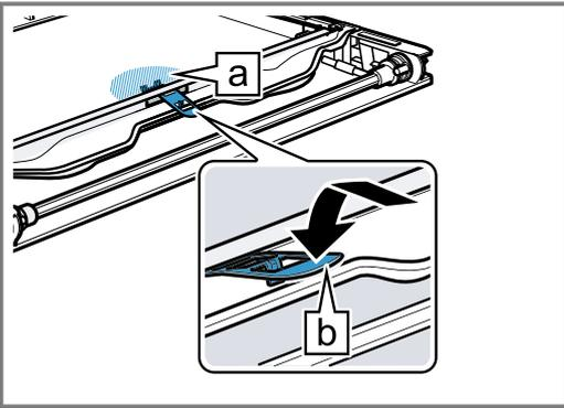
6. Place the inner pane onto the appliance door so that the number **a** is legible at the bottom right. Insert the inner pane into the fixing rail **b** at an angle towards the back.
