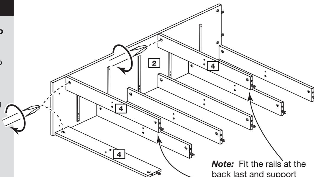
**Note:** Fit the rails at the back last and support them until the left side has been fitted in the next step.
