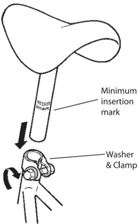
\* Under no circumstances should the seat post project from the frame beyond its Minimum Insertion mark. If your seat post projects from the frame beyond these markings, the seat post or frame may break, which could cause you to lose control and fall.
