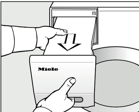
■ Remove the condensed water container.
