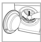
Check the vent tube and any permanent venting fixture to make sure that there has been no accumulation of fluff or lint. Remove lint that collects around the filter and the outlet vents.
