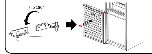
Tip: If there are 'O' rings on the hinge after flipping, remove them before installing the door.
