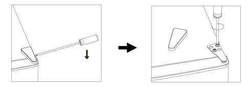
2. Remove the hole caps that are on the top left of the unit and fix them to the opposite side.
