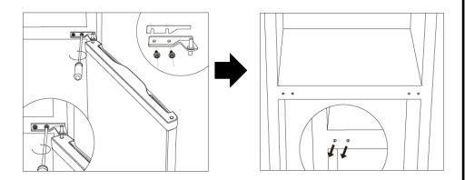
4. Remove the hinge plug from the top of fridge door and fix it to the opposite side.
