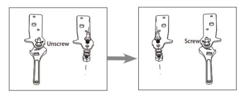
6. Place the fridge door on to the bottom hinge. Flip over the middle hinge (by 180°) and put the bottom pin of the middle hinge into the top of the fridge door and screw the middle hinge back onto the opposite side of the appliance. You must ensure the fridge door is aligned horizontally and vertically, so that the seals are closed on all sides before finally tightening.
