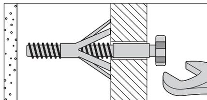
For use when fitting or supporting heavy loads such as shelving, wall cabinets and coat racks.
