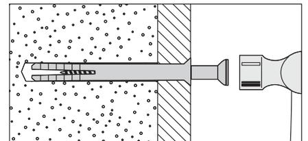
For use with walls stuck with plasterboard. The hammer fixing allows it to be fixed to the wall rather than the plasterboard. Always check the fixing is secure to the retaining wall.
