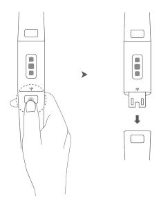
• Installing the strap: Clip in the strap from the correct ends and directions.
