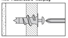
For use when attaching light loads on to plasterboard partitions.
