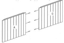
3. Assemble the three bath panels together by locating the metal dowels into the holes of the centre panel (B).
