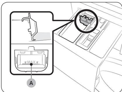
First insert the provided liquid detergent guide in the **II** **main-wash compartment**. Then, apply liquid detergent to the guide below the marked **max line (A)**.
