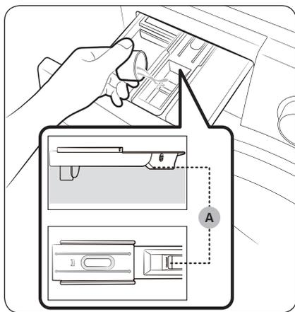
3. Apply fabric softener to the **III softener compartment**. Do not exceed the **max line (A)**. Softener is dispensed into the wash during the final rinse.
