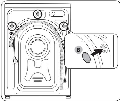
3. Insert the **bolt caps (B)** to the holes (marked with circle in the figure).
