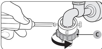
4. Insert the adaptor onto the water tap, and then tighten the screws while lifting the adaptor.
