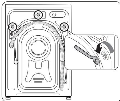
1. Locate the shipping bolts (marked with circle in the figure) on the rear side of the washing machine.
