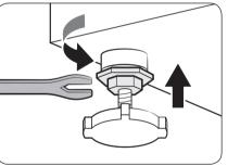
**3.** When levelling is complete, tighten the nuts using the spanner.
