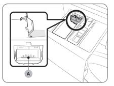
First insert the provided liquid detergent guide in the **1 main-wash compartment**. Then, apply liquid detergent to the guide below the marked **max line (A)**.
