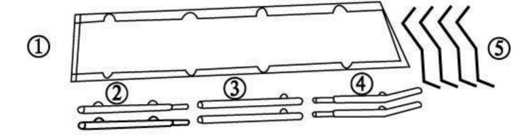
STEP 1. ASSEMBLE 3 PIECES TOGETHER FOR EACH SIDE RAIL.
