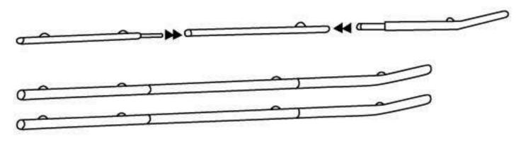
STEP 2. PUSH SIDE RAILS THROUGH THE SIDES OF THE COVER.
