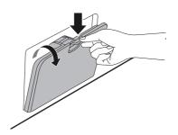
Remove the drain plug from the drain tube first, and then drain the water.
