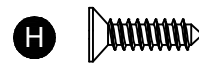
H 4 x 15mm Screw x 16 SCR04015M (With extra few pieces for spare)
