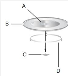
A-glass tray; B-hub (under); C-turntable shaft; D-turntable ring
