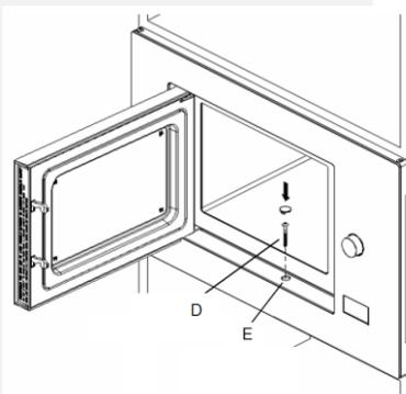
5. Open the door, fix the oven to the cabinet with screw (D), at the installation hole.
