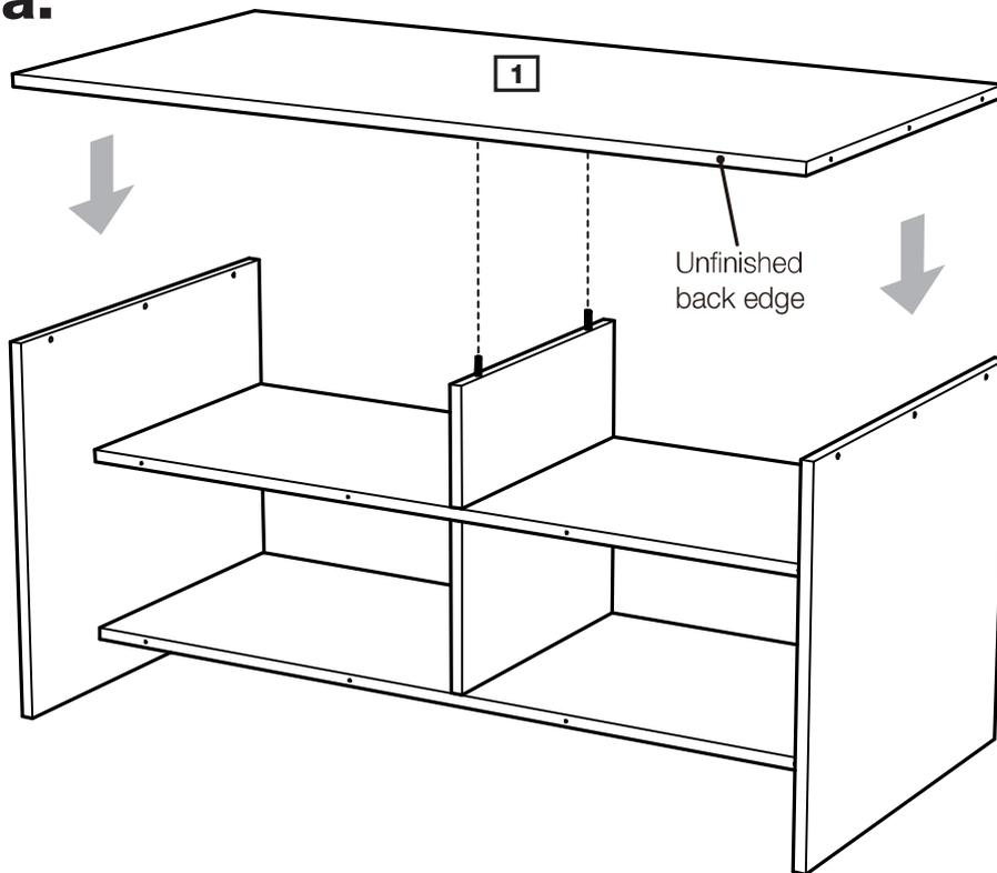
**b:** Use Screws **D** to fix Top panel **1** onto the unit.
