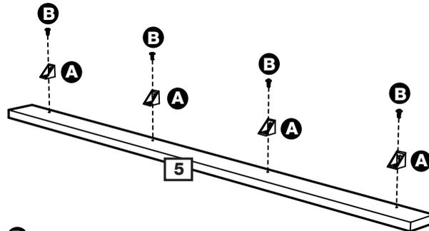
**b:** Position the Front panel **5** onto the Bottom panel **2** using Screws **B**.
