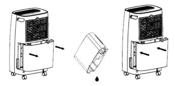
**Note:** Do not remove the float from the water tank. The water full sensor will no longer be able to detect the water level correctly without the float and water may leak from the water tank.
