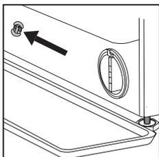
Remove the stopper of the “emergency drain hose” at the end of the hose and let the water flow into the container.
