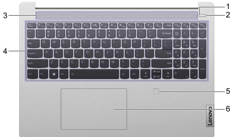
Figure 3. Base view-for 16-inch models (IdeaPad Slim 5 16AHP9, IdeaPad Slim 5 16IMH9, and IdeaPad Slim 5 16IRU9)
