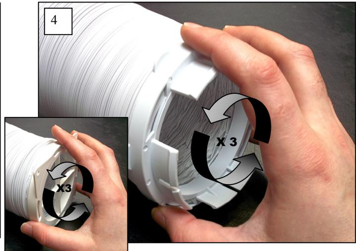
One end of the vent hose is fitted with an adaptor which can be pushed into the exhaust outlet at the bottom rear of the tumble dryer. The free end should be led to a suitable outlet. It may simply be hung through an open window or a more permanent connection made using the four holes in the adaptor flanges.
