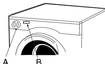
**A. THE TIMER** Turn the timer knob fully clockwise before selecting the required drying time based on the recommendations on the control panel.
