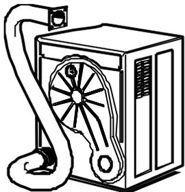
**Note: Do not obstruct or add a mesh to the vent hose outlet during use and ensure that it cannot be blocked or bent sharply which may obstruct the air flow. It is recommended that the interior of the hose be periodically inspected and cleaned if necessary.**
