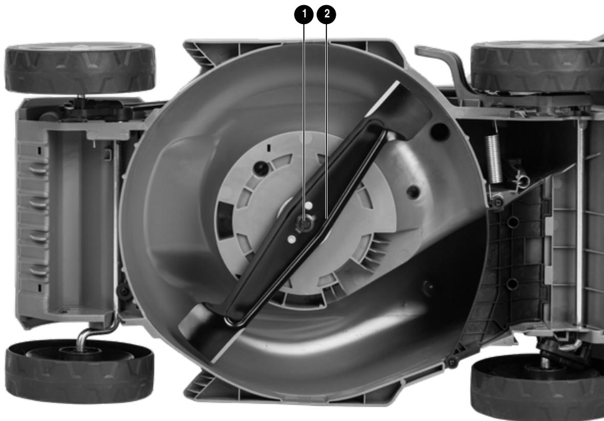
Turn the machine carefully onto its right side and inspect the blade. If blunt or damaged, replace it.
