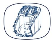
iii. Lift up the rear flap before assemble the grass bag.Hang the collection bag on the mower.
