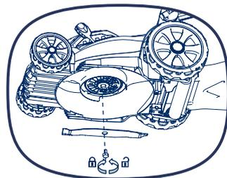
**NOTE: Replace this cutting device after 50 hours mowing or 2 years whichever is sooner regardless of condition. If the cutting device is cracked or damaged, immediately replace it with a new one.**
