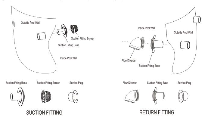
Please Note: The Black Rubber gasket (Fitting Gasket) should always be slid over the threaded plastic suction or return fitting and be on the inside before the fitting is placed through the pool wall to make a watertight connection.
