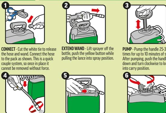
**CONNECT** - Cut the white tie to release the hose and wand. Connect the hose to the pack as shown. This is a quick couple system, so once in place it cannot be removed without force.
