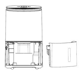
Step 1: Remove the water tank.
