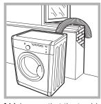
The end of the hose must be facing downwards, in order to prevent the hot, damp air from forming condensation in the room or the tumble dryer.
