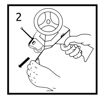
Feed tape between guide and roller, sticky side down
