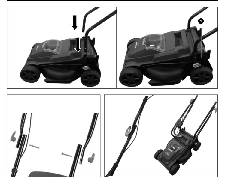
Insert the left and right lower handles into the slots of the housing. Ensure the locking pin button (1) is secured into place.
