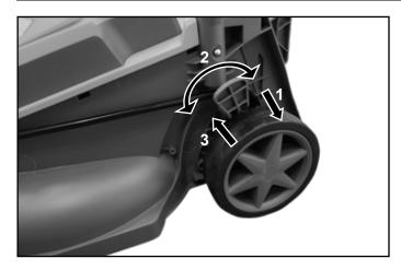
IMPORTANT! Set the cutting height only when the motor is switched off and the isolator key has been removed.
