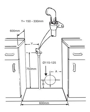
The illustration shows the minimum space required by the dryer and the position of the gas wall connector. It is not acceptable to use a forward facing mounting plate because of the space limitation. The sideways facing assembly must be used and this should be fitted so that the flexible hose hangs down from the bayonet connector.
