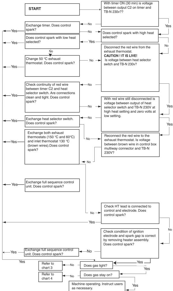
Chart 3. Motor runs Full Sequence Control produces ignition sparks, but gas does not ignite.
