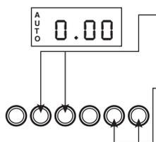
**Step 5** With the Cook Period & End Time buttons still held in, press either the "+" or "-" buttons to set the correct time of day.
