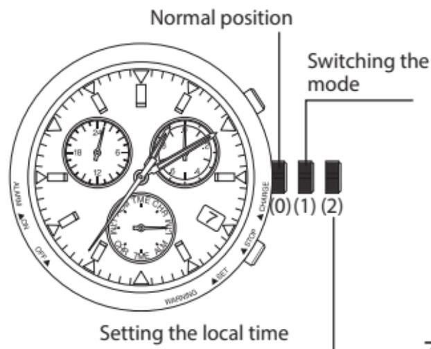
3. Rotate the crown to the left (counterclockwise) or right (clockwise) to adjust the desired time difference (hours only).
