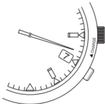
If the watch stops due to insufficient charge, be sure to fully charge it, perform the all reset and 0-positioning procedure and then re-set the time as well as the calendar.
