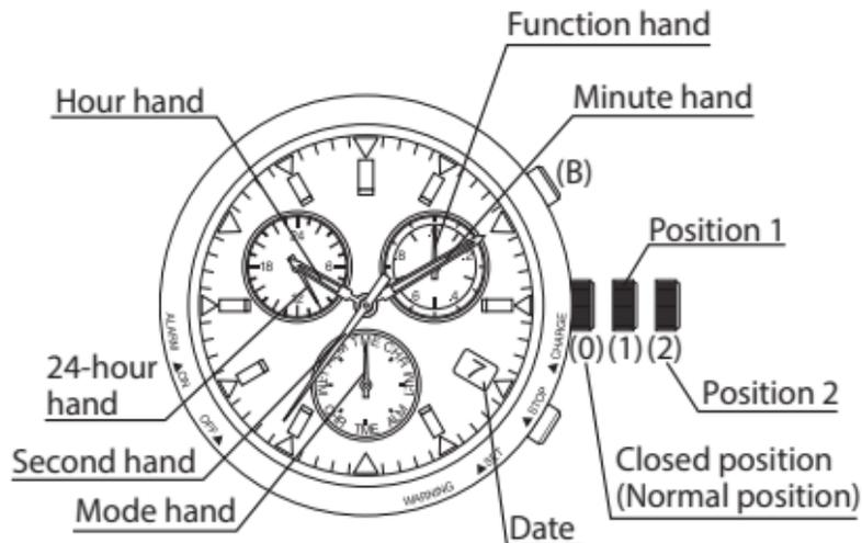
2. Pull the crown out two steps to position 2 (time adjustment position) and press the upper right button (B).
