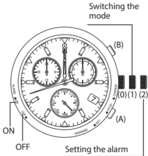
3. Rotate the crown to adjust the time to when the alarm should sound.
