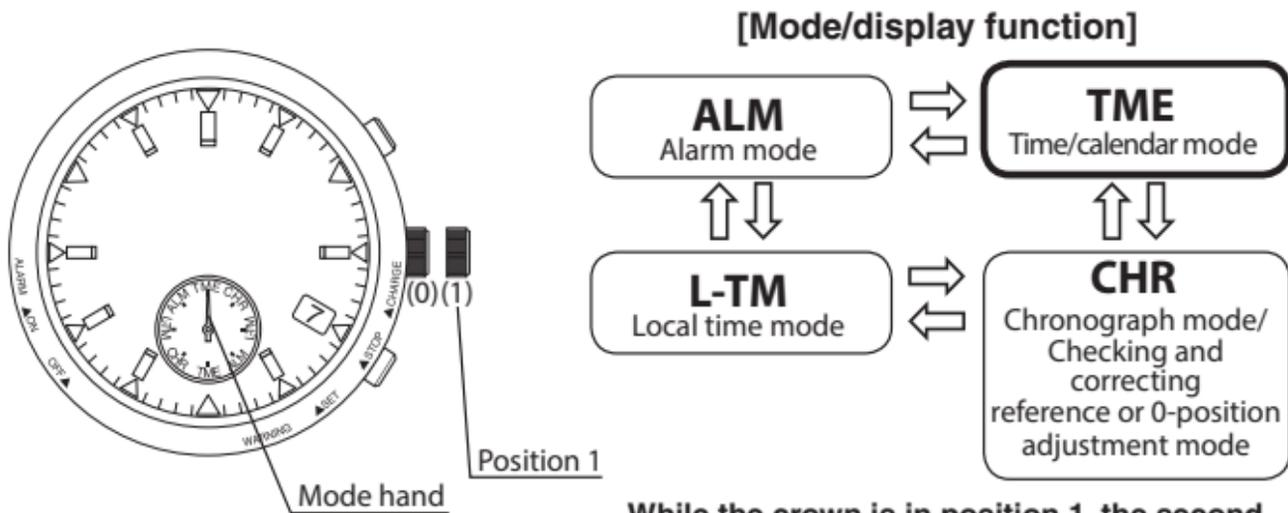
**While the crown is in position 1, the second hand points to the 30 seconds position.**
