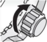
Push the crown in to the case. With gentle pressure towards the case, rotate the crown clockwise to secure it to the case. Be sure to tighten firmly.<br>A line drawing of a watch crown with a curved arrow pointing clockwise, indicating the direction to rotate it to lock it. |
