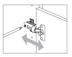
**C:** To move doors left or right: loosen screw shown and move doors to suit.
