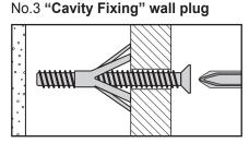
For use with plasterboard partitions or hollow wooden doors.
