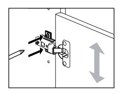
**b:** To move doors in or out: loosen screw shown and move doors to suit.
