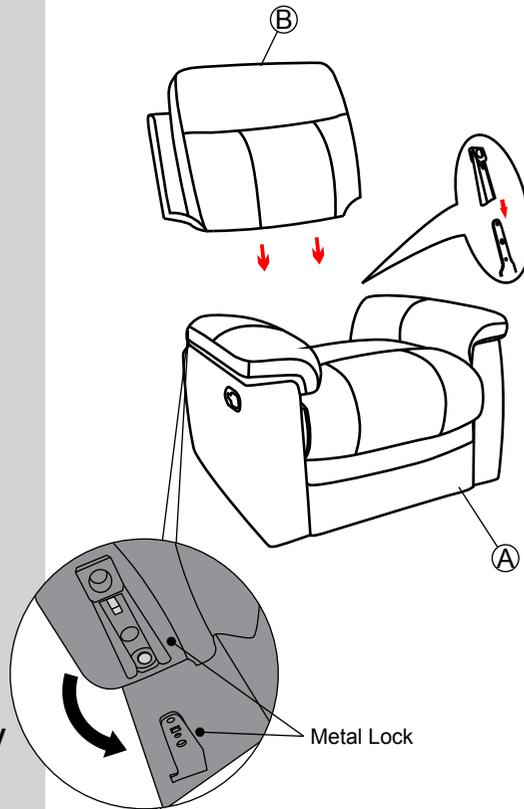
**NOTE:** Carefully line up the two side metal locks. Ensure they align correctly.
