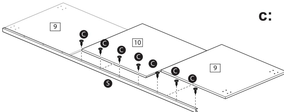
**d:** Mount door handle **S** on segment **9** with 4x screws **C** and on middle segment **10** with 3x screws **C**.
