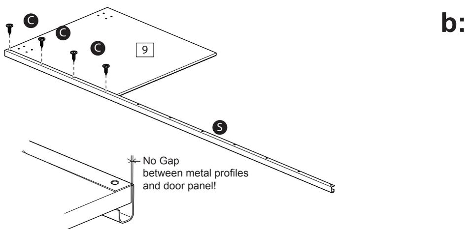
**c:** Mount segment middle **10** with 3x screws **C** on door handle **S**. Mount segment **9** with 4x screws **C** on door handle **S**.
